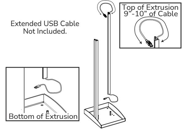
Prior to installing Upright Extrusion route USB Extended USB cable into extrusion. Leave 9-10" of cable at the top of the extrusion.
