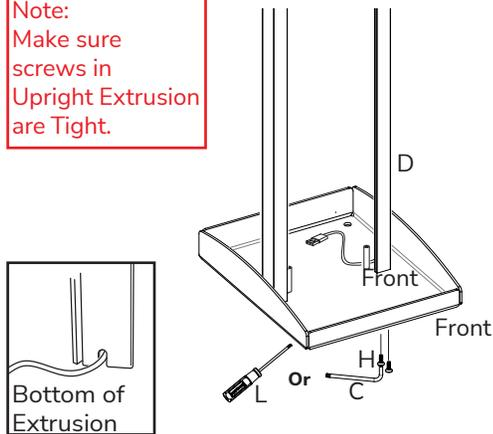
Install the Upright Extrusion (D) using M5X20mm Flat Head Torx Screws (H) tighten using T-25 Torx Wrench (C).
