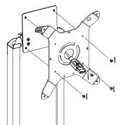
Tablet Enclosure mounts to 100mm mounting pattern. Use M4 x 8mm Button Head Phillips (I) to attach Enclosure.
