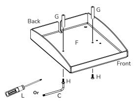
Install the two Round Spacers (G) using two of the M5 x 20mm Flat Head Screws (H) tighten using T-25 Torx Wrench.
