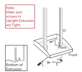
Install the Uprignt Extrusion (D) using M5X20mm Flat Head Torx Screws (H) tighten using T-25 Torx Wrench (C).
