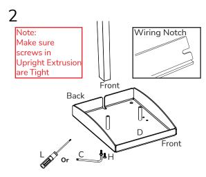
Locate the Upright Extrusions (D). Make sure extrusion has the flat edge facing forward. Install the M5 X20mm Flat Head Torx Screws (H) tighten using T-25 Torx Wrench (C).
