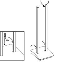
Secure Base Cover with M5 X 20mm Flat Head Torx Screw (H) using T-25 Torx Wrench(C). 8
