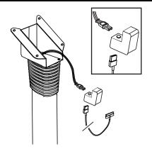
Installation of Recommended C7 Power Cord to iPad USB 30 Pin Power Adapter.
