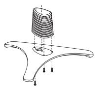
D - #8-16 x 1/2" Pan Head Phillips Self Threading Screw.
